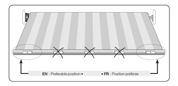
**NOTE:** Prior to October 1<sup>st</sup>, 2022, the wind sensor back plate was affixed to the front bar with a strip of double-sided tape. Since then, we have decided to screw the back plate into the front bar to ensure it doesn't fall off.
