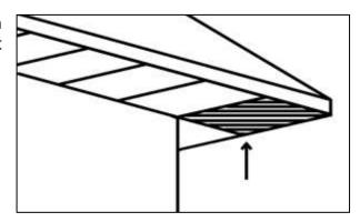
This means that your awning cannot be wider than the wall, even if the eaves are wider than the wall and you had planned the installation under eaves.
