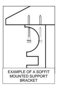
**ATTENTION!** You must securely fasten all the screws to the rafters. Some constructions may require more lag bolts. **WHEN IN DOUBT**, consult a certified contractor. The improper installation could cause the awning to collapse and cause injury and property damage.
