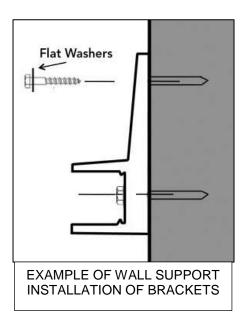
**WARNING!** You must make sure that masonry bolts are securely fastened into holes. Otherwise, remove them and consult a hardware store for appropriate masonry bolts.
