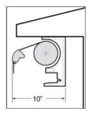
**WARNING!** Proper positioning of the cornice supports is the most important and critical step in erecting the awning. It is imperative that all screws are well anchored to the rafters or other major structural elements.
