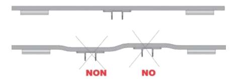
You will need to install shims if the brick surface is uneven.
