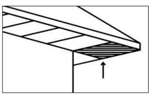
This means that your awning cannot be wider than the wall, even if the eaves are wider than the wall and you had planned the installation under eaves.
