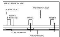
The shims can be installed on top of the siding if a sufficiently large surface is in direct contact against a solid surface. Otherwise, the shims can be installed underneath the siding where a hole can be cut into the siding for the shim to be inserted.
