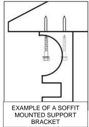
**ATTENTION!** You must securely fasten all the screws to the rafters. Some constructions may require more lag bolts. **WHEN IN DOUBT**, consult a certified contractor. The improper installation could cause the awning to collapse and cause injury and property damage.
